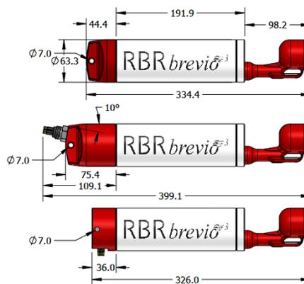
**RBR*brevio*<sup>3</sup> dimensions with three different battery end-caps**
