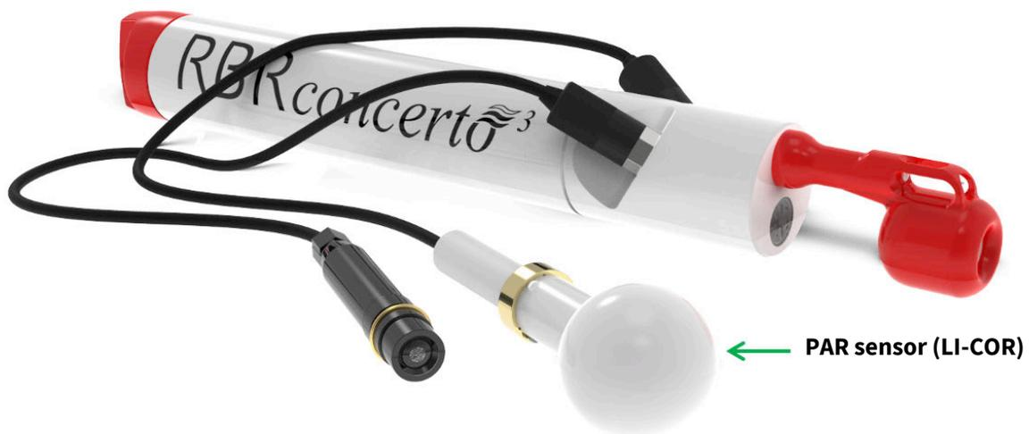
**RBRconcerto<sup>3</sup> C.T.D.DO.PAR with a spherical PAR sensor (LI-COR)**
