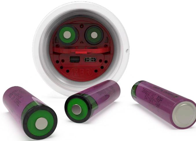
**RBR standard instrument with batteries removed**
