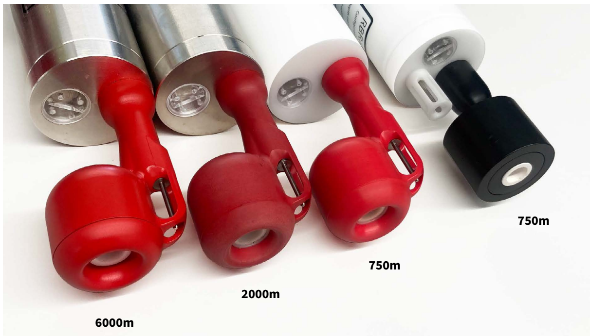
750m-, 2000m-, and 6000m-rated conductivity cells
