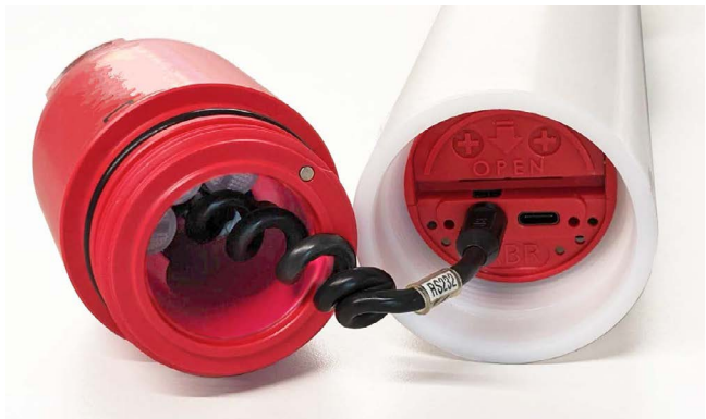
Open instrument with a connectorised end-cap
