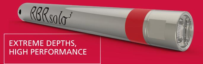
The RBRsolo<sup>3</sup> T|deep, RBRsolo<sup>3</sup> D|deep, and RBRduet<sup>3</sup> T.D|deep in titanium housing are small but highly durable. Deployable to the bottom of the Marianas Trench, they provide accurate and stable measurements in the most challenging environments. Low power consumption allows for extended schedules.
